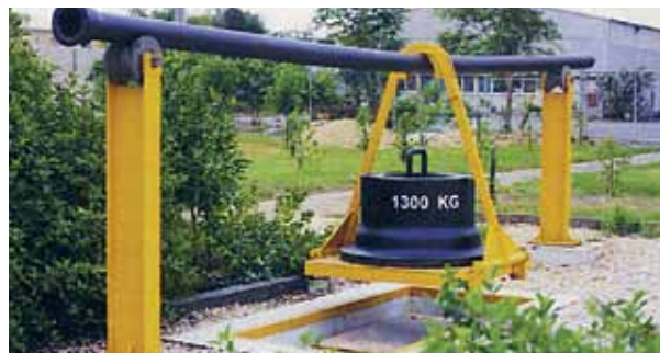
Deformation of a small DN pipe under external loading.
