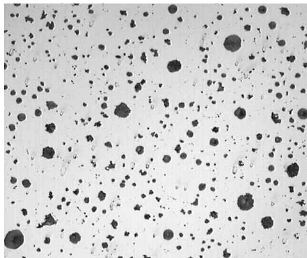
In ductile iron the graphite particles appear as small spheres, eliminating any risk of crack propagation. The material is no longer brittle. It is strong and ductile.
