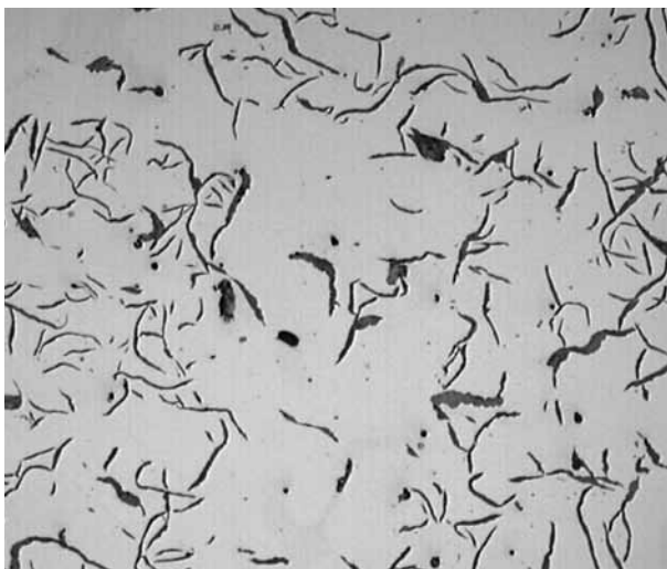
In the previously used Grey Iron the carbon was present in flake form, rendering the material brittle.
